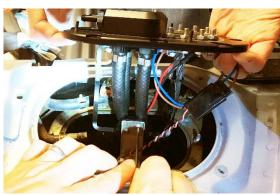
24. Continue to lower and rotate the assembly until the Radium collector box sits properly into the OEM gas tank baffle.
