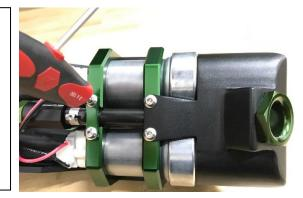
20. Secure the fuel temperature sensor ring terminals to the "TEMP" studs on the underside of the top plate using the lock nuts. There is no polarity so they cannot be criss-crossed.
