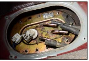
5. To detach the SAE quick disconnect lines, simply squeeze the locks and pull the fitting away from the metal tube. Reinstall the plastic lock to the fitting. To detach all other hoses, use pliers to release the spring clamps and pull the hoses off. Use a rag to clean up any spilled fuel.
