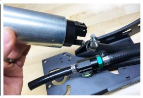
18. Reinstall the clamps using the 4 screws. The pump(s) will hang from the bottom, as shown.
