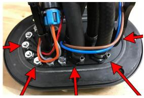
23. NOTE: The level sender cannot be attached until the hanger assembly is halfway installed into the gas tank. This step MUST be performed with 2 people (Installer#1 and Installer#2). First, remove the 2 small M4x0.7mm screws from the hanger bracket using a 2.5mm Allen hex wrench. Then, while outside the gas tank, plug in the connector with blue and brown wires to the level sender connector that was assembled in earlier steps.
