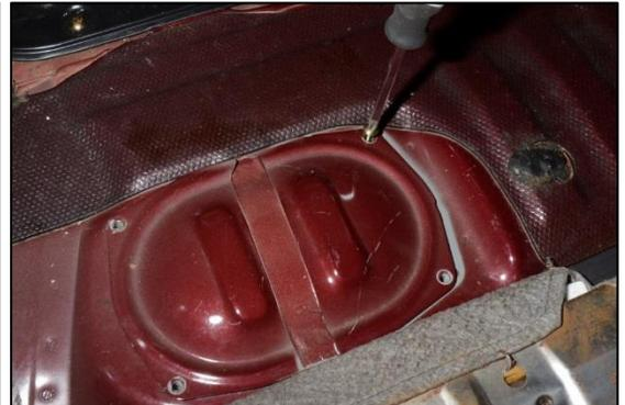
2. Once removed, it is recommended to clean the top of the fuel pump housing and the surrounding area. This will prevent loose dirt from falling into the gas tank.
