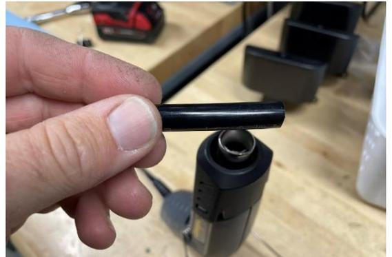
17. As shown, secure the hose/tube using one of the provided EFI hose clamps.
