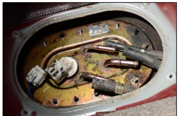
5. To detach the SAE quick disconnect lines, simply squeeze the locks and pull the fitting away from the metal tube. Reinstall the plastic lock to the fitting. To detach all other hoses, use pliers to release the spring clamps and pull the hoses off. Use a rag to clean up any spilled fuel.
