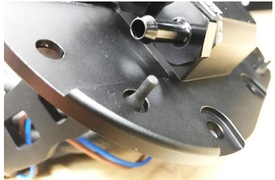
22. From the underside of the top plate, be sure that the OEM gasket is seated in the machined lip, as shown.
