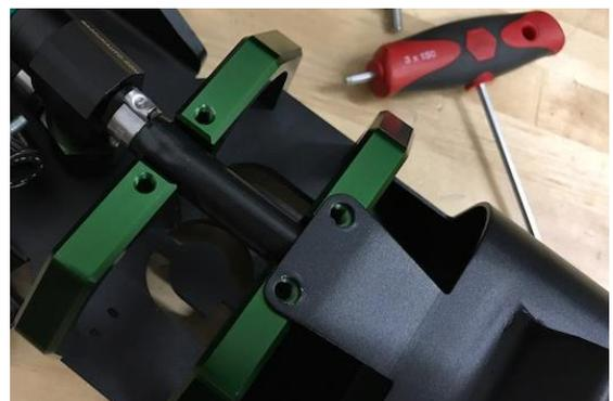
14. From the backside of the assembly, remove the two outer M5 bolts using a 3mm Allen hex wrench. Detach the collector box from the assembly, as shown.
