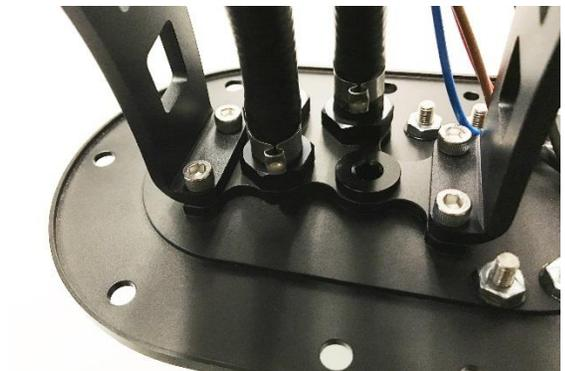
13. To install the fuel pumps, first remove the four M5 bolts in the areas shown using a 3mm Allen hex wrench.
