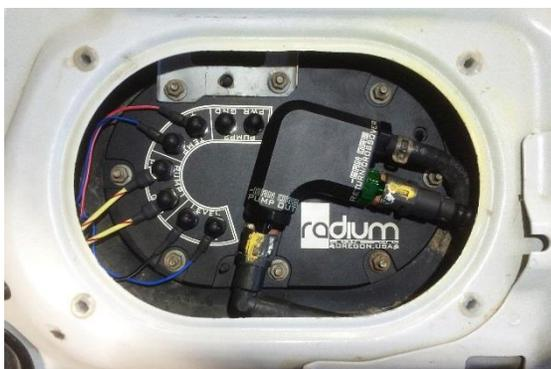
28. As shown, there are many wire color variations for all of the model years. Referencing the pinout chart, insert the ring terminals onto the corresponding studs.
