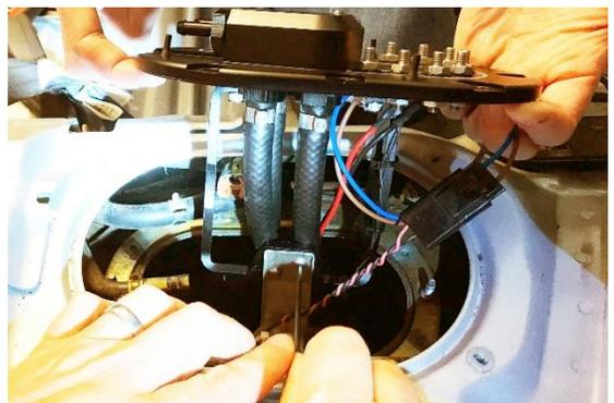
24. Continue to lower and rotate the assembly until the Radium collector box sits properly into the OEM gas tank baffle.
