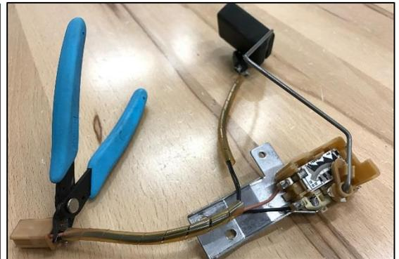
8. For the fuel level sender, first twist the wires together for flexibility.
