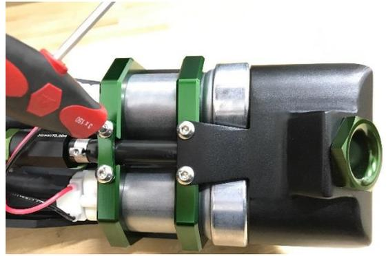
20. Secure the fuel temperature sensor ring terminals to the "TEMP" studs on the underside of the top plate using the provided lock nuts and 3/8 nut driver. There is no polarity so they cannot be criss-crossed. Extra nuts may be present in the kit and can be used as spares.
