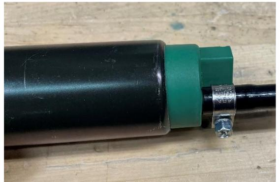
18. Reinstall the clamps using the 4 screws. The pump(s) will hang from the bottom, as shown.
