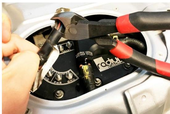
27. Use the large diameter shrink tube and large AWG ring terminals to connect the pump power wires. The connection points on the hanger are labeled "PWR" for positive and "GND" for negative. Shown at right is a 2006-2007 Subaru (with the SAE fuel return connection).
