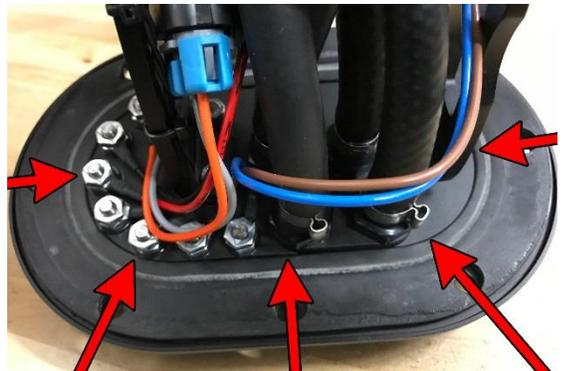
23. NOTE: The level sender cannot be attached until the hanger assembly is halfway installed into the gas tank. This step MUST be performed with 2 people (Installer#1 and Installer#2).
