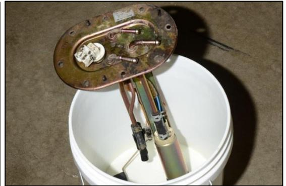
6b. NOTE: Subaru changed from external post-pump filters to internal post-pump filters around 2005 (depending on the model). This filter is easily identified as it is mounted directly to the fuel pump outlet, as shown.
