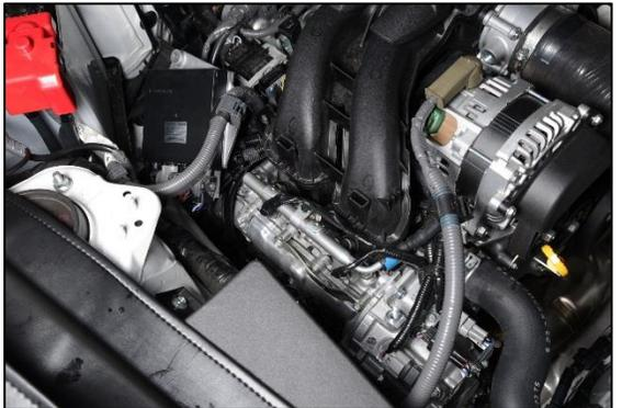
4. Set the new Radium bracket in place. Using a 12mm socket wrench, secure using the two OEM M8 bolts.
