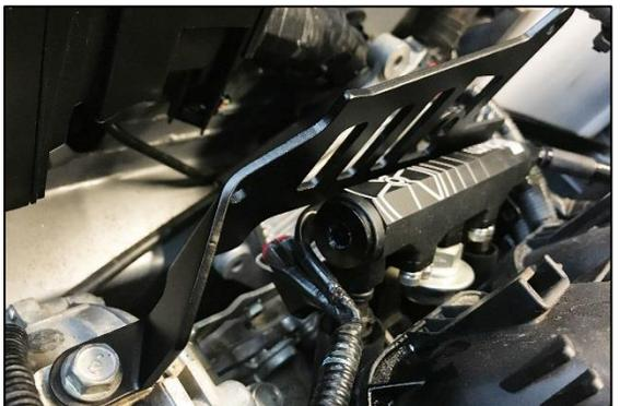
5. Using a 4mm Allen hex wrench and 10mm socket wrench, lineup the direct injection ECU and secure the top and front holes using the provided M6 button head screws and nuts.
