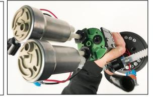
11. Rotate the fuel pump(s) so the power wires are facing outwards. Next, lubricate the orange connector seal(s) and plug in the fuel pump connector(s), as shown.
