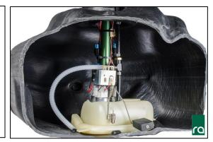
30. To reinstall the OEM black hold-down ring, rotate clockwise and tighten. NOTE: The top 3 fittings can freely swivel for additional space.
