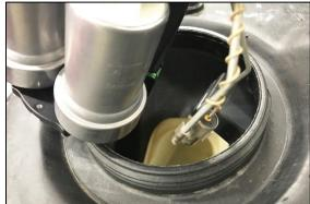
27. Next, insert the end of the loose convoluted tubing into the rear opening of the gas tank, as shown.
