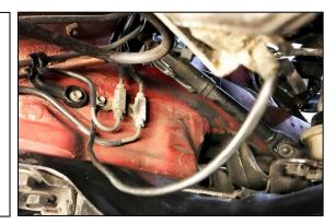
63. NOTE: for this plumbing kit to connect properly, the fuel rail (not included) must have an 8AN ORB threaded front port. Radium Engineering recommends, 2JZ-GTE Fuel Rail P/N: 20-0215. Install the included 8AN ORB to 10AN male fitting to the front port of the fuel rail.
