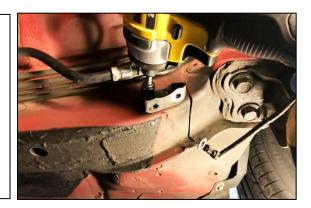
49. From the engine bay, remove the fuel rail feed line banjo bolt.
