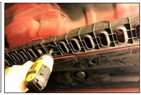
51. Pry the locking tabs to release the plastic hard line covers.
