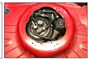
2. To depressurize the fuel system, first squeeze the tab and unplug the gray wiring connector on top of the pump housing (shown).
