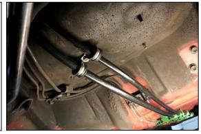
71. Using the provided cable zip ties, secure the return line to the retainers, as shown.
