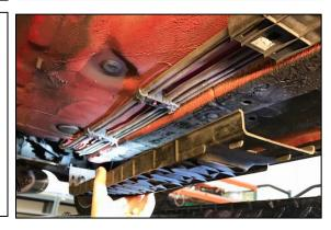
53. Using a 10mm socket wrench, remove the last plastic cover that is located to the left rear of the differential near the muffler.
