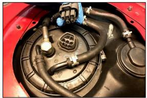
3. Disconnect the OEM banjo bolt fitting using a 17mm wrench. Using pliers, dislodge the OEM spring clamps and pull off the fuel return and vent hoses. Use a rag to clean any spilled fuel.
