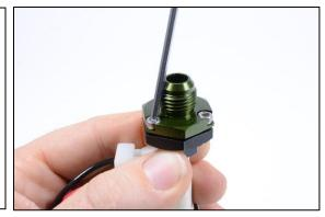
10. For single or dual fuel pump applications, block-off the unused ports on the underside of the triple pump block using the included 6AN ORB plug fittings. For clearance purposes, it is best to plug the hole nearest the fuel sensor mount (shown).
