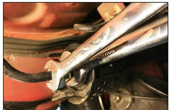
4. Using a 10mm socket wrench, remove the ground wire ring terminal bolt. NOTE: This could be found on any one of the 3 bolts shown.
