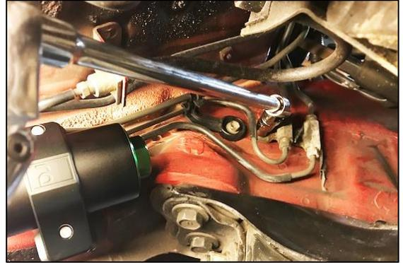
11. Relocate and secure the electrical ground wire ring terminal to the mounting boss, as shown.
