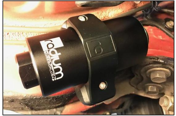
10. Using a 10mm socket wrench, remove the M6 bolt that secures the brake line adapter junction point shown.
