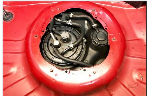
2. To depressurize the fuel system, first squeeze the tab and unplug the gray wiring connector on top of the pump housing (shown).
