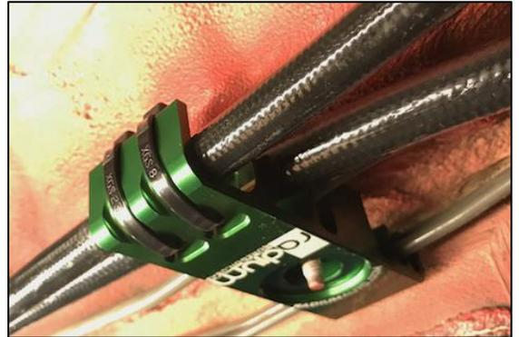
11. NOTE: the rearmost retainer may not require zip ties as the retainer touches the floorboard.
