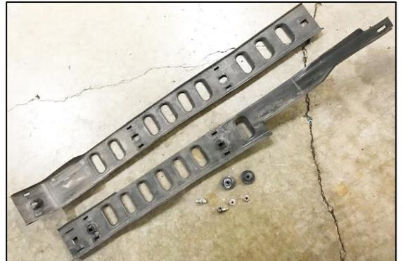
7. Carefully pry and pop off the 4 hard line retainers, as shown.
