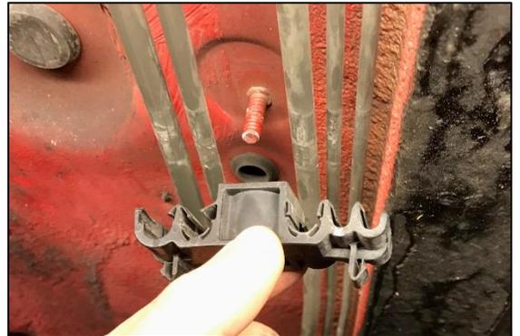
8. Note: There are a few different types of hard line retainers in the MKIV Toyota Supra. Some are shorter than others. For instance, the JZA80 chassis has raised M6 nuts in some locations.
