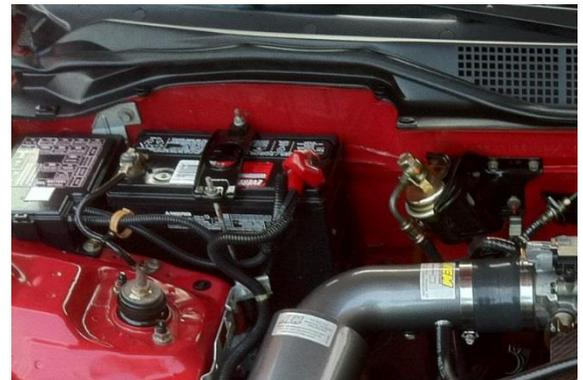
2. Disconnect the feed hose and fuel pressure regulator (FPR) return hose. Catch all spilled fuel. Using a 10mm socket wrench, remove the 2 FPR bolts. These will not be reused. Carefully remove the FPR and do not lose the sealing O-ring.
