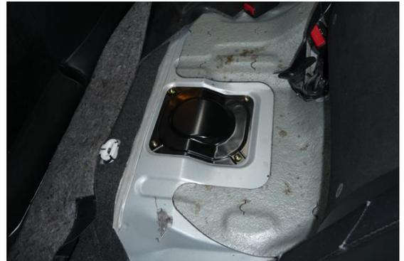
2. To depressurize the fuel system, first squeeze the tab and unplug the gray wiring connector on top of the pump housing (shown). Start the engine and allow it to stall. Remove the key from the ignition. Unscrew the gas tank filler cap temporarily to relieve any residual pressure.
