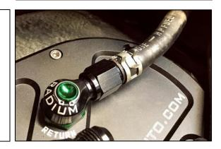
54. Turn the ignition key to the ON position to pressurize the fuel system. Confirm the new fuel pump(s) are properly operating. Check for leaks. If no leaks are found, start the vehicle.
