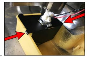
37. During acceleration, the check ball will open supplying the lift pump with ample fuel located inside the OEM sub tank as shown.
