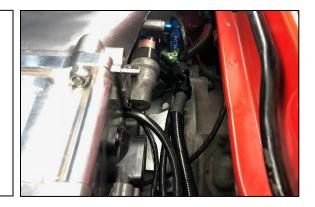
12. Replace the plastic fuel line cover. Some modification and tweaking of the cover will be required to fit the 8AN feed line.
