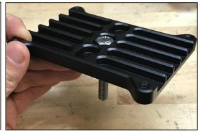
3. Fit the mounting plate to the bottom of the fuel filter housing. Using a 5mm Allen hex wrench, secure with the four short M6 bolts.
