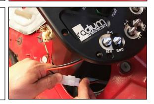
43. To install into the gas tank, the fuel level float must enter the gas tank first. Carefully tip the fuel hanger assembly to angle in the fuel level float, as shown.
