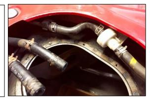
34. Plug in the 2-wire extension harness with the white connector to the lift pump. Lower the baffled lift pump assembly into the gas tank as shown.
