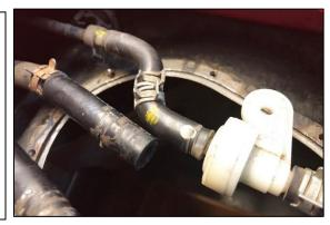
33. Rotate the rubber vent hose 180 degrees and secure with the spring clamps, as pictured.
