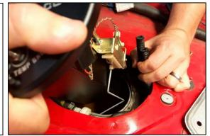
44. Find another person to help with this step as it is difficult. The fuel level sender will need to be pressed inward with an object to get it past the gas tank opening.
