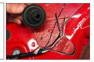
49. The OEM fuel pump power wiring will be reused for the lift pump. The OEM wiring does NOT need to be upgraded since the lift pump operates at very low pressure thus low current.
