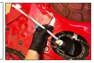
35. To secure the baffle into the OEM sub tank, it is important that all 4 tabs are installed properly. First, tilt the baffle up and push the baffle to the rear of the tank. With a flashlight confirm the 2 rear tabs are locked into place.
