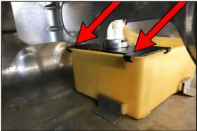
36. Next, gently squeeze the side walls of the OEM sub tank to allow the 2 baffle tabs to lock in place.
