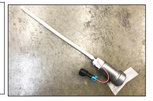
27. Insert the pump through the bottom side of the included lift pump baffle. NOTE: depending on the pump, it may save time to place one of the included worm drive clamps on the bottom side prior to inserting the pump.
