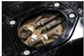
3. Before proceeding, it is recommended to clean the top of the fuel pump housing and the surrounding area. This will prevent loose dirt from falling into the gas tank.
