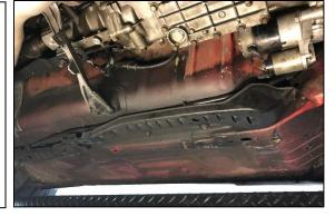
13. At the fuel pump hanger, connect the feed line from step 7 onto the feed port swivel fitting on the feed port. When tightening the hose end, hold the swivel fitting with an adjustable wrench.
