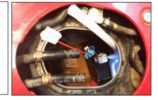
40. Insert the M5 socket head bolt through the black ground wire ring terminal and fuel level/temperature sensor assembly. Secure to the FST canister rivet nut using a 4mm Allen hex wrench.
