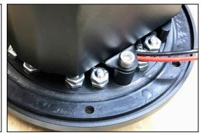
31. From the top side of the plate, pull the 4 rubber nubs up. They will lock into place.
