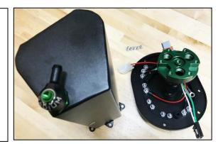
9. Using a 1" wrench, unscrew the upper hex of the female 10AN coupler, as shown.
