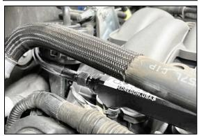
13. Shown is the LH rear fuel rail port when using the 20-1435 plumbing kit. This side of the engine will use the shorter PTFE hose provided in the kit. Note how the 90 degree hose end attaches to the banjo fitting which point towards the center of the engine. This permits the necessary flexibility when connecting this short hose to the nearby OEM feed line.
