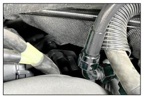
14. Follow this procedure for connecting the 6AN male adapter (provided in the plumbing kits) to the SAE quick connect fuel feed line on the firewall.
