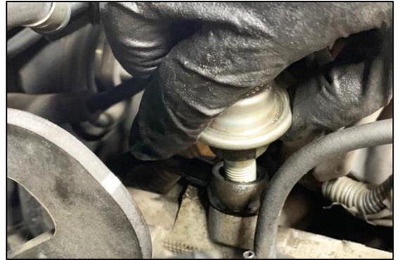
32. If using the 20-0371-PK Plumbing Kit, the banjo fuel feed line will not be reused. This can be unbolted from the engine block or simply pushed out of the way as shown. If elected to keep it in the engine bay, blow the fuel out with compressed air.
