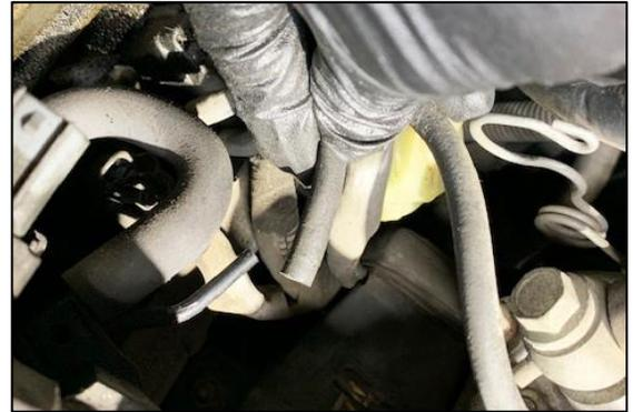
22. Dislodge the spring clamps and pull off both throttle body coolant hoses.
