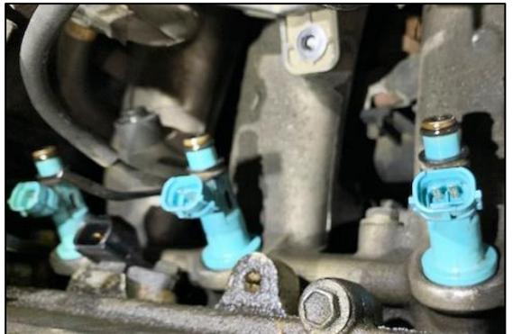
39. Lineup and place the fuel rail down on the engine. Fully seat the upper O-ring of the fuel injectors. NOTE: it is normal for the front of the fuel rail to be in slight contact with the engine harness cover, as shown.
