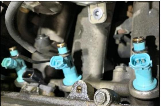
39. Lineup and place the fuel rail down on the engine. Fully seat the upper O-ring of the fuel injectors. NOTE: it is normal for the front of the fuel rail to be in slight contact with the engine harness cover, as shown.
