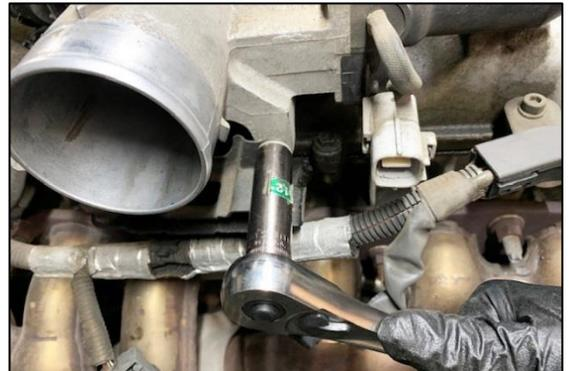
18. Remove the 2 lower throttle body bolts using a 12mm socket wrench. Remove the throttle body bracket.
