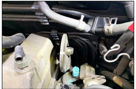
33. Using a 12mm wrench unscrew the three M8x1.25mm fuel rail bolts.
