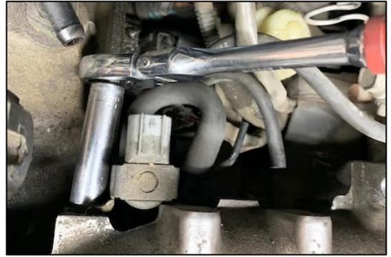
16. Using pliers dislodge the two spring clamps and remove the PCV valve hose from the vehicle.
