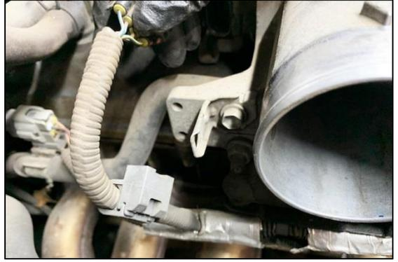
11. Unplug the throttle body motor connector.
