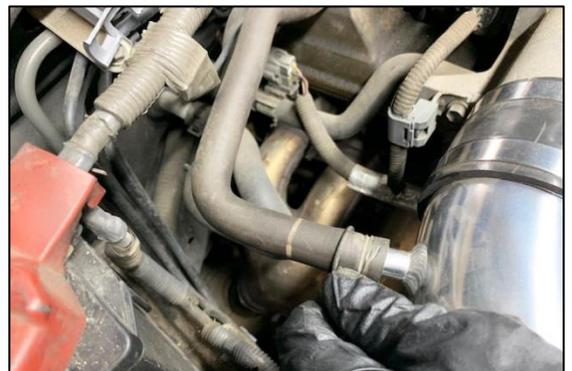
5. Using pliers, remove the vent valve hose from the intake pipe.
