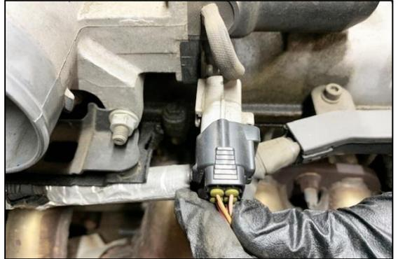
12. Using needle nose pliers, dislodge the plastic wiring harness stay just under the throttle body.
