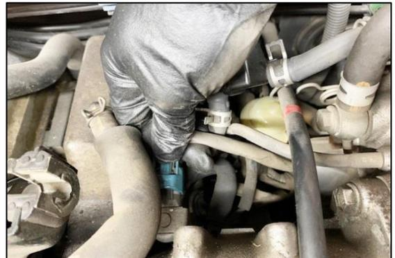
14. Remove the hose from the EVAP purge solenoid shown.
