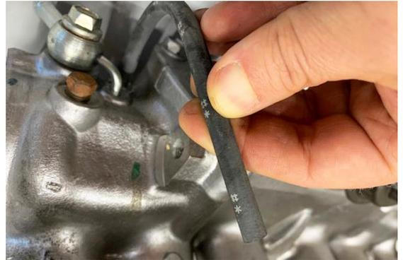
42. Insert the provided vacuum hose to the fuel pulse damper barb. The included "Y" fitting will be required if tapping into an existing vacuum hose.
