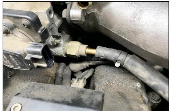
23. Remove the ACIS solenoid vacuum hose shown.
