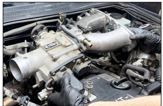
25. Using a 10mm socket wrench, unscrew the two ACIS actuator mounting bolts.
