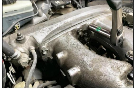
21. Remove the vacuum hose from the lower intake runners, as shown.
