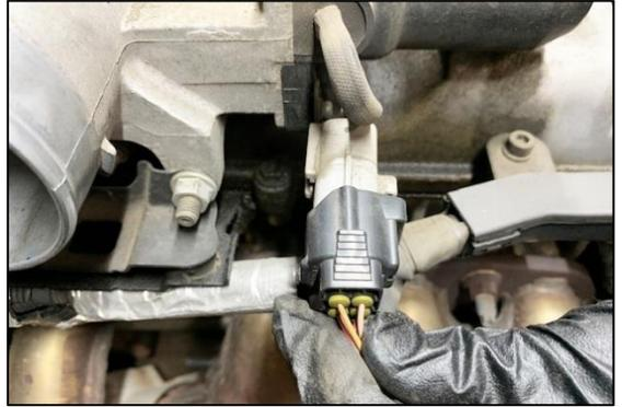
12. Using needle nose pliers, dislodge the plastic wiring harness stay just under the throttle body.
