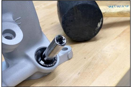
**37. Lubricate all adapter fitting O-rings and secure to the four 8AN ORB ports.**
