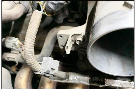
11. Unplug the throttle body motor connector.
