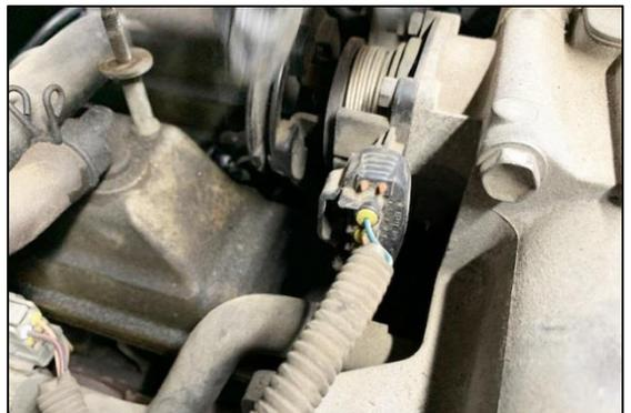
10. Using a flat blade, dislodge the wiring harness connection near the throttle body.
