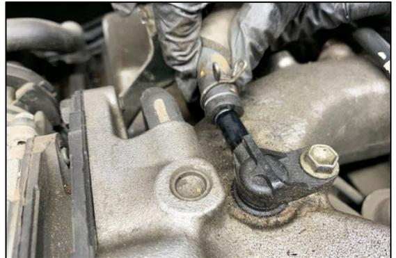
17. Remove the 2 upper throttle body bolts using a 12mm socket wrench.
