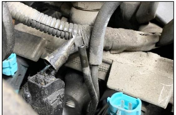
28. Unplug the camshaft position sensor.
