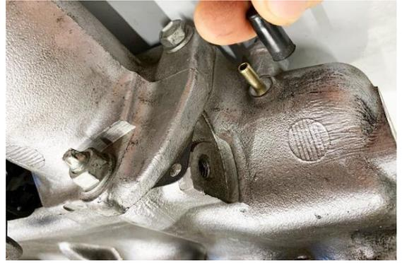
41. Another option for fuel pulse damper vacuum reference (for the 20-0371 plumbing kit) is this source pictured.
