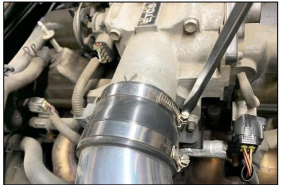
7. As shown, remove the throttle cable adjustment screw using 14mm wrenches.
