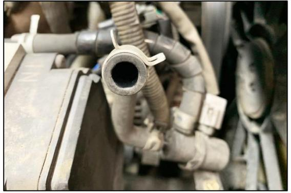
6. Remove the intake pipe from the throttle body.
