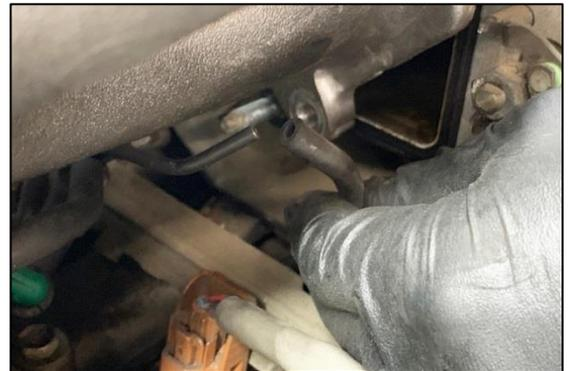
24. Carefully pull the intake manifold assembly upwards to remove.
