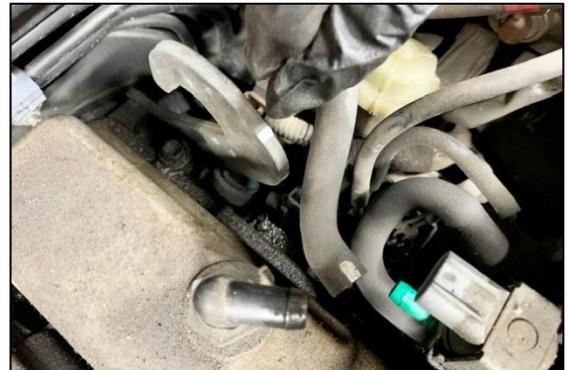
15. Remove the EVAP purge solenoid M6 bolt shown using a 10mm socket. Allow the solenoid to freely move. Removal is not necessary.
