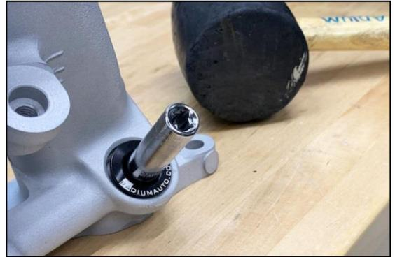
**37. Lubricate all adapter fitting O-rings and secure to the four 8AN ORB ports.**
