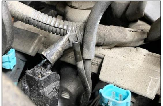
28. Unplug the camshaft position sensor.
