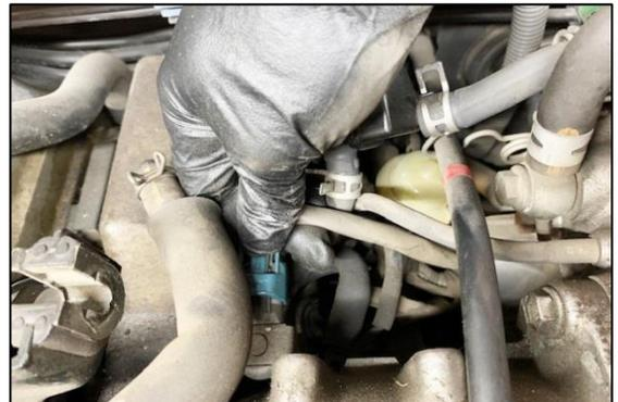
14. Remove the hose from the EVAP purge solenoid shown.
