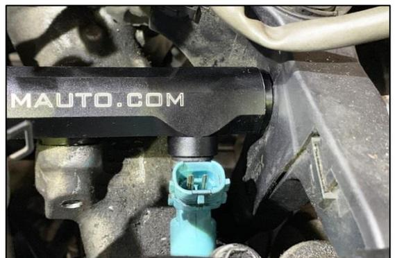
40. For the 20-0371-PK plumbing kit, find a good vacuum source for the fuel pulse damper. Many 2JZ-GE engines use a vacuum cap on the vacuum port shown. This is one option for the vacuum signal.
