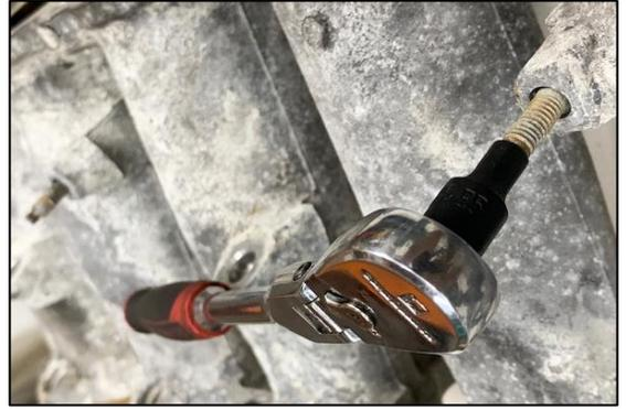
31. Using a 22mm wrench, remove the fuel pulse damper mounted to the fuel feed banjo. Have a rag handy as fuel will spill from this connection.
