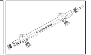
8. Press the small end of the spacers (YELLOW) into the underside of the rail mounts, as shown. Place the small washers (RED) under the bolt heads (BLUE). Insert the bolts through the fuel rail and spacers. Roll the O-ring (GREEN) up the bolt threads.
