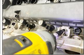
4. Carefully pull the fuel rail assembly away from the cylinder head to dislodge. The fuel injectors should remain attached to the fuel rail. Place on a workbench and catch any fuel that drips out.
