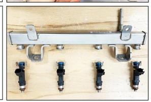
6. The 4 OEM fuel injector locking clips will be reused.
