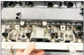
5. One by one, carefully unclip the fuel injectors from the OEM fuel rail, as shown.
