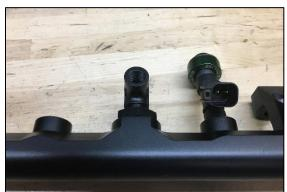
79. Using the same PTFE paste and tightening procedure as the first 1/8NPT elbow, install the second elbow into the outlet of the first elbow, as shown.
