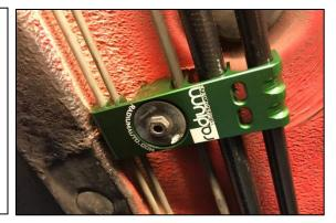
70. Just in front of the LH half shaft, the OEM hard lines make tight bends. For optimal fuel flow, the replacement PTFE fuel lines will bypass this potential restriction.
