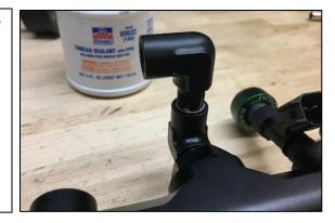
80. When the tightening is complete, the second elbow fitting should be pointing at approximately 45 degrees to the fuel rail, as depicted.
