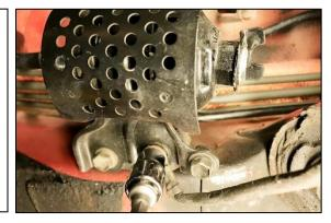
47. Using a 10mm socket wrench, remove the 2 bolts that secure the fuel filter to the fuel filter mount.
