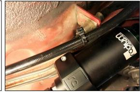
69. Using the OEM hardware and a 10mm socket wrench, install the 4 Radium retainers.
