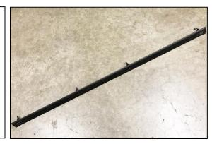
32. Using 10mm wrenches, remove the gas tank shield. This piece is held in by 6 bolts.
