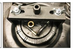
4. Before removing the OEM unit, place an empty bucket nearby as there will be residual fuel in the gas tank. Slowly lift the assembly straight up.
