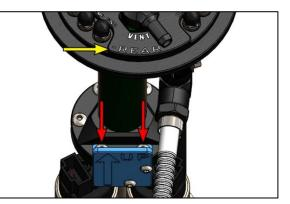
24. Find the 3 sensor wires hanging from the fuel hat. Match each wire color and push each terminal into the OEM 3-pin connector (see yellow arrow pictured).
