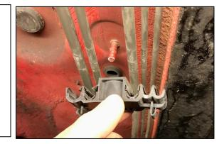
55. In one piece, pull the fuel feed line out of the vehicle. This will include everything from the fuel pump hanger banjo soft line to the fuel filter inlet inverted flare hard line, as shown.
