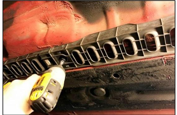
51. Pry the locking tabs to release the plastic hard line covers.
