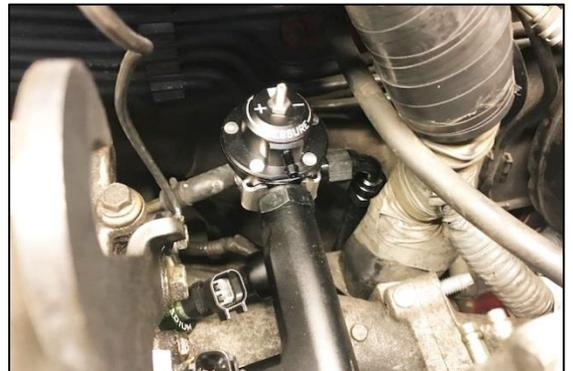
68. Secure the return line near the fuel filter using one of the provided cable zip ties, as shown.
