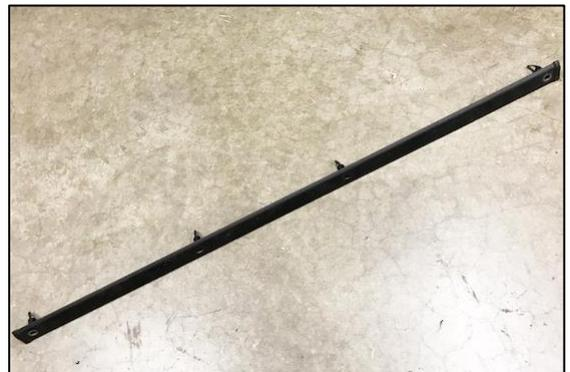
32. Using 10mm wrenches, remove the gas tank shield. This piece is held in by 6 bolts.
