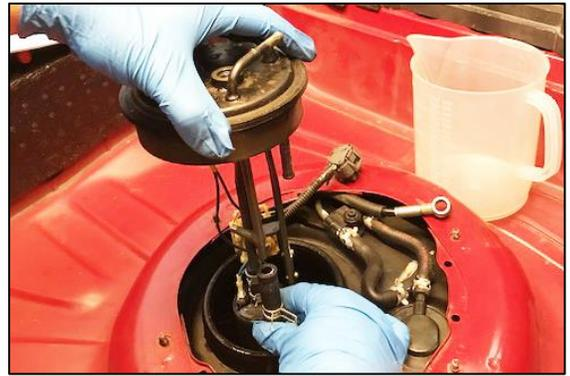
5. As shown, there are 2 versions of the OEM Toyota Supra fuel pump assembly. The main difference is with the internal fuel return line.
