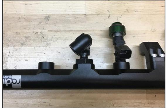
81. Apply a small amount of PTFE paste to the pressure gauge threads and install into the elbow fitting, as shown. Use a 7/16" wrench to tighten the gauge and a second wrench to hold the elbow fitting.
