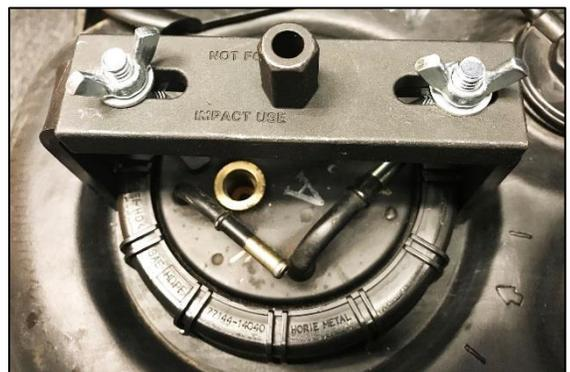
4. Before removing the OEM unit, place an empty bucket nearby as there will be residual fuel in the gas tank. Slowly lift the assembly straight up.
