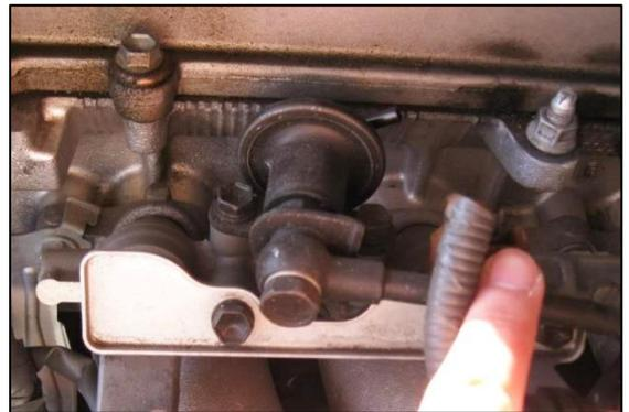
57. **NOTE: The long OEM return hard line does not HAVE TO be removed from the vehicle.**
