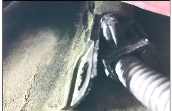
36. From above, dislodge the connector tabs and flip up. Cut all wires as close to the connector as possible. Remove some of the electrical tape and strip the wire insulation back 1/4", as shown.
