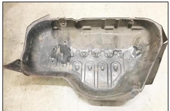
33. Using 10mm wrenches, remove the exhaust muffler shield. This piece is held in by 3 bolts.
