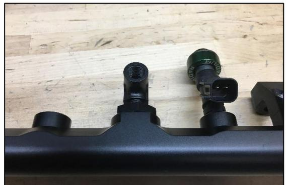
79. Using the same PTFE paste and tightening procedure as the first 1/8NPT elbow, install the second elbow into the outlet of the first elbow, as shown.
