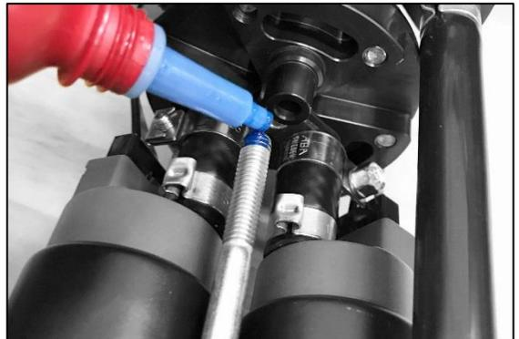
18. If installing 1 or 2 fuel pumps, screw in the bolt (shown red) with a 10mm socket wrench just enough before the filter assembly becomes crooked. Do NOT tighten! Use the included filter support bracket (shown blue) and the screws (shown yellow) to keep the assembly straight.
