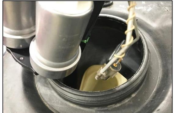
27. Next, insert the end of the loose convoluted tubing into the rear opening of the gas tank, as shown.
