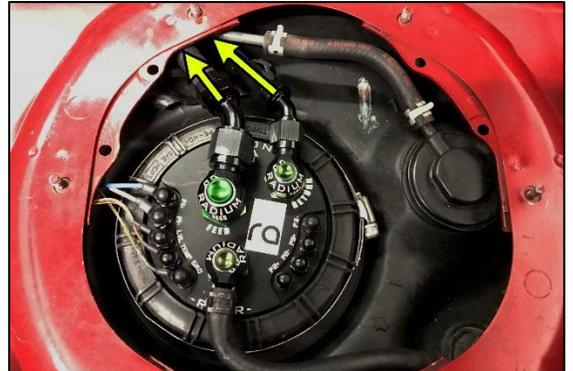
67. For this plumbing kit, the fuel pressure regulator (not included) must have a 6AN male return port. Radium Engineering recommends, DMR P/N: 20-0223-0X which can connect directly to the rear port of the Radium fuel rail. Line up the long return hose to the FPR and cut to length.
