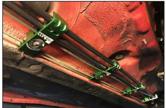
73. After tightening all related fittings, secure the fuel filter clamp using a 4mm Allen hex wrench. Notice how the filter is slide upwards inside the clamp to add ground clearance.
