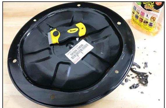
43. Find the adhesive foam included in the kit. Peel the backing off and apply on the flat areas around the cover on the inside of the 6 mounting holes (shown in blue). Cut to length.
