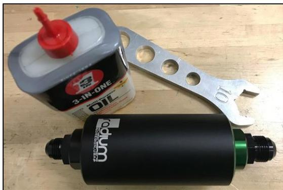
60. Place the fuel filter on the lower half mount with the outlet facing the engine bay and the inlet facing the rear of the vehicle.
