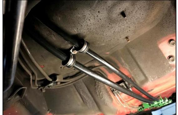
71. Using the provided cable zip ties, secure the return line to the retainers, as shown.
