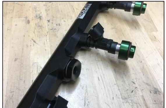
77. Apply a conservative amount of PTFE paste to the male threads of one of the 14-0332 1/8 NPT elbows and screw it into the 14-0119 adapter.
