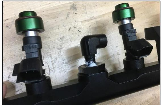
78. NPT threaded fittings should first be tightened finger tight. Then, using a wrench, add another 1.5 to 3 turns until fully tight and pointing straight up (same direction as the injector electrical connections).
