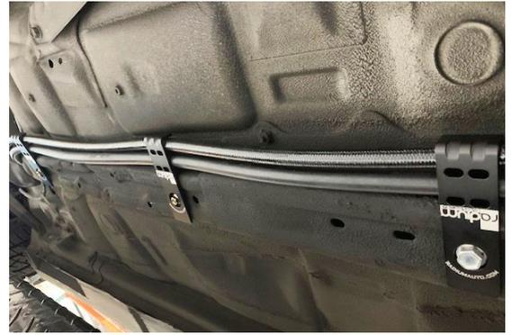
6. Fasten the hoses under the car near the transmission using the provided clamp and a 15mm socket, as shown.
