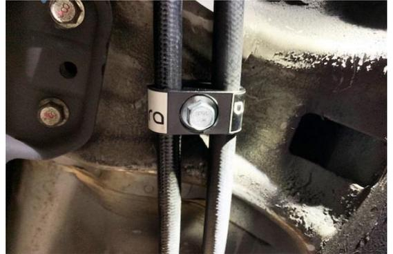
7. Route the 2 fuel hoses up in front of the fuel tank so they can be accessed from the LH access panel inside the vehicle.
