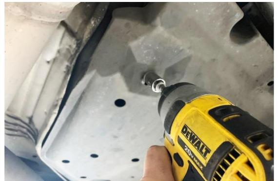
3. Temporarily remove the protective shield from the vehicle.
