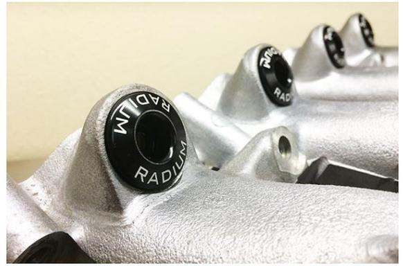
6. Position the fuel rail in place making sure all injectors are lined up properly in the Radium injector seats. Next, press firmly on the fuel rail to seat the injectors' lower O-rings.
