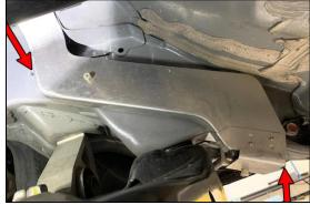
12. Install the fuel filter bracket assembly over the top of the heat shield using the OEM bolts.
