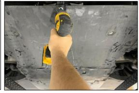
7. A small flat head screwdriver and 10mm socket wrench will be required to remove all associated fasteners for the skid plate (shown).
