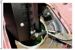
27. Reinstall the OEM M5 flange nuts using an 8mm wrench. Tighten to factory specs in steps using an alternating crisscross pattern.
