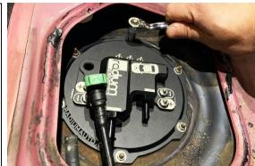
28. Lubricate the "PUMP OUT" SAE quick connect and push the OEM feed line in. Push down the OEM green lock to secure the connection. Gently tug the hose connection to verify a positive lock has been made.
