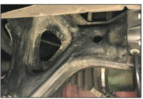
7. Slide the long M8 bolt on the filter mount through the hole in rear subframe. Install the M8 washer and locking nut. Use a 13mm socket wrench, but do not torque the nut yet.
