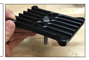
5. Fit the mounting plate to the bottom of the fuel filter housing. Using a 5mm Allen hex wrench, secure with the four short M6 bolts.
