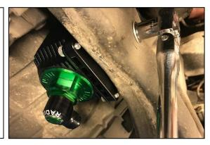
8. Double check that all connections are tight. Prime the fuel pump until system pressure is achieved then check for leaks. Address any possible leaks and re-test.
