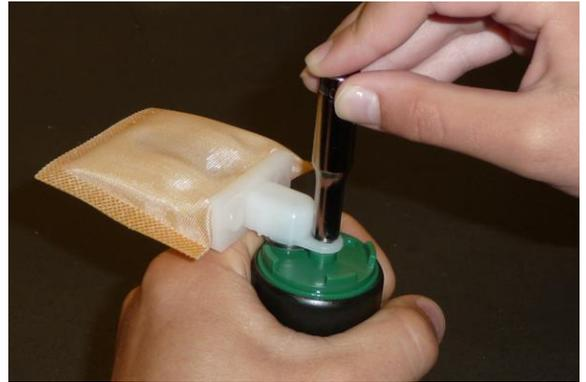
22. Locate the 2 sections of heat shrink in the kit and slide them over each BMW female spade terminal.
