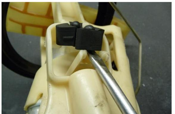
10. Take note of the clocking orientation of the plastic holder in respect to the fuel pump's outlet barb. To release the BMW fuel pump, pull the plastic tabs downward (as shown). The holder will come out the bottom of the pump.
