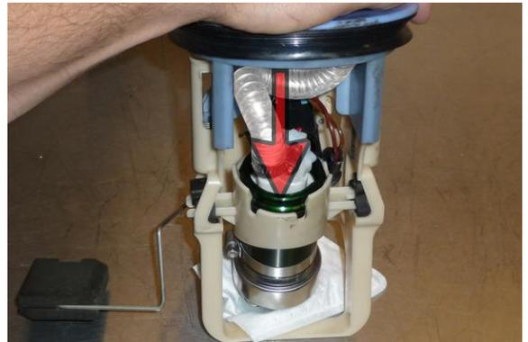
24. Be sure the gasket is installed before reinstalling into the tank.
