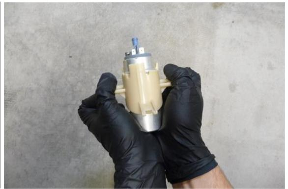
11. Before connecting the electrical wires, understand how the spade terminals lock into place. There are holes in the male terminals. These are visible on the OEM fuel pump terminals, as shown.
