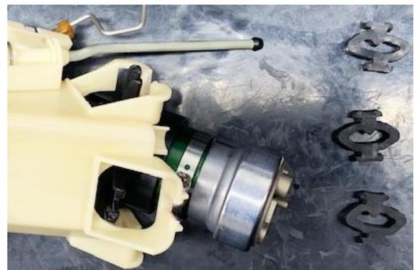
20. From the outside, push the 3 rubber grommets inwards to secure the fuel pump to the OEM unit, as shown.
