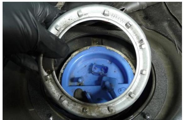
25. Connect the battery and turn the key to the ON position. Listen for the new fuel pump to confirm the electrical was performed properly and check for fuel leaks. If no leaks are found, start the vehicle. The engine may run rough for a few seconds until the air is bled from the system.
