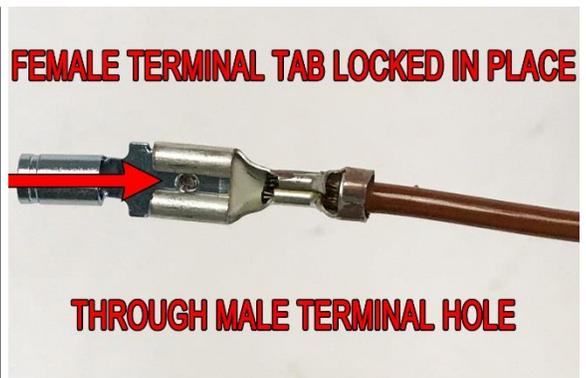
15. If using a Walbro F90000262 Fuel Pump, no adapter wiring harness is required as it uses the same terminals (shown) found on the BMW fuel pump. Skip to Step 18.
