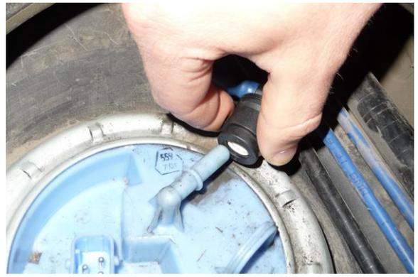
6. To unfasten the ring connection, BMW sells a special tool, P/N: 16 1 020. If not available, a rubber mallet hammer and punch will suffice. When spinning the ring counterclockwise a dab of glue will break free. If the ring is stubborn, get a second person to hit the opposing side of the ring simultaneously.
