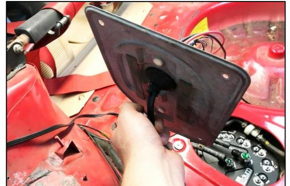
62. Use the large diameter shrink tube and large gauge (AWG) ring terminals to connect all fuel pump wires.
