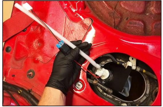
45. To secure the baffle into the OEM sub tank, it is important that all 4 tabs are installed properly. First, tilt the baffle up and push the baffle to the rear of the tank. With a flashlight confirm the 2 rear tabs are locked into place.
