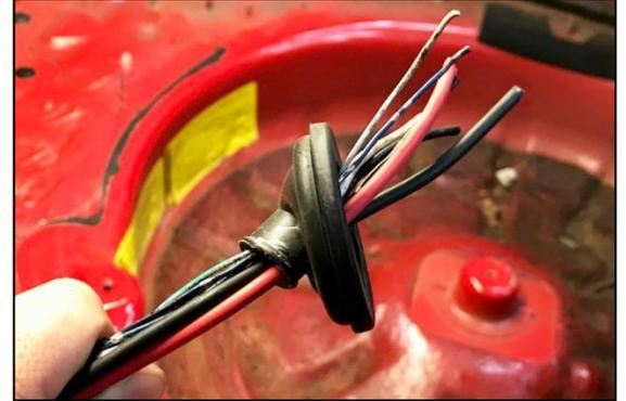
61. Reattach the rubber grommet to the OEM fuel tank access cover. Allow ample slack for terminating the wires in the following steps.
