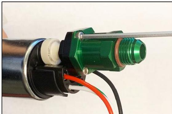
24. After tightening all bolts evenly, inspect the internal side of the green fitting. When installed properly, the plunger should be slightly sticking out of the center hole at rest, as shown.
