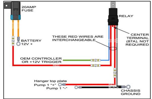
60. Once the new unterminated FST fuel pump wires are assembled, run them through the OEM rubber grommet along with the unterminated OEM wires.
