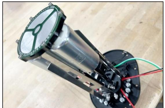
33. If using brushed pumps, plug in the fuel pump connectors.
