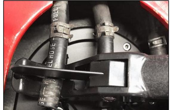
66. Push the OEM hoses onto the barb and secure with the OEM spring clamps, as shown.
