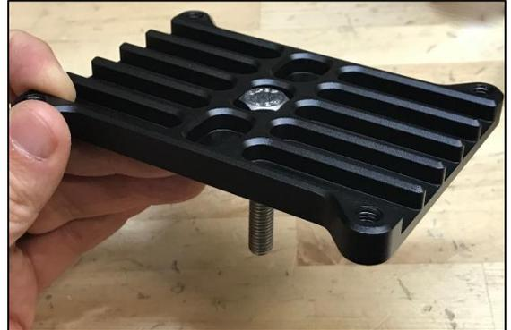
3. Fit the mounting plate to the bottom of the fuel filter housing. Using a 5mm Allen hex wrench, secure with the four short M6 bolts.
