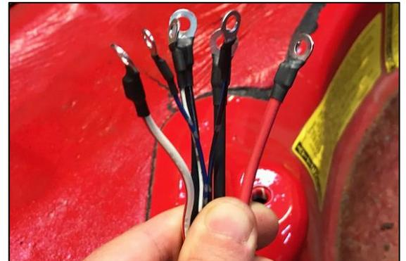
63. Referencing the chart, secure all ring terminal connections to the electrical studs using the provided acorn nuts and an 8mm socket wrench. Do NOT overtighten.
