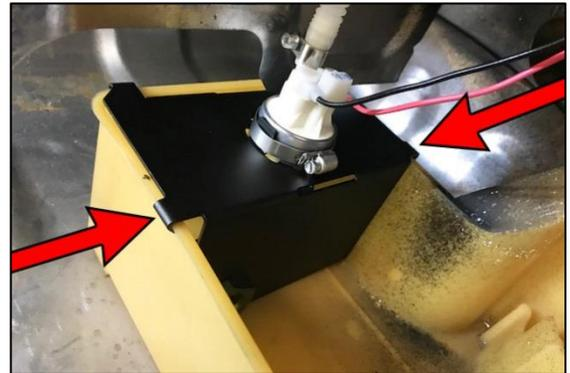
47. During acceleration, the check ball will open supplying the lift pump with ample fuel located inside the OEM sub tank as shown.
