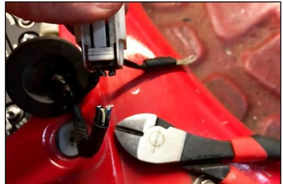
57. Cut the OEM external ground terminal off using diagonal cutters, as shown.
