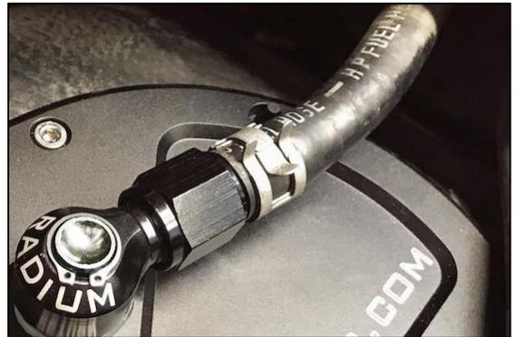
64. Turn the ignition key to the ON position to pressurize the fuel system. Confirm the new fuel pump(s) are properly operating. Check for leaks. If no leaks are found, start the vehicle.
