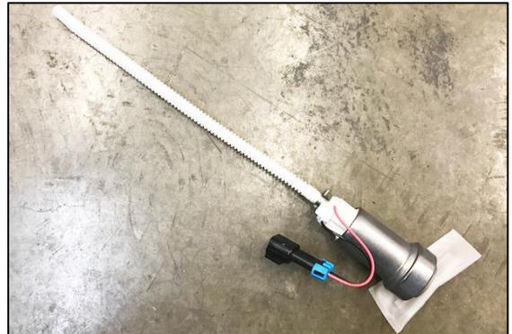
37. Insert the pump through the bottom side of the included lift pump baffle. NOTE: depending on the pump, it may save time to place one of the included worm drive clamps on the bottom side prior to inserting the pump.
