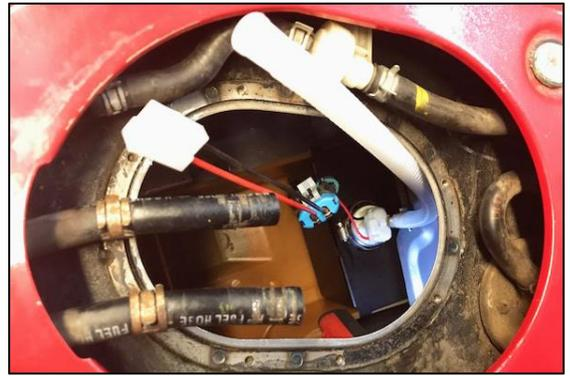
50. Insert the M5 socket head bolt through the black ground wire ring terminal and fuel level/temperature sensor assembly. Secure to the FST canister rivet nut using a 4mm Allen hex wrench.
