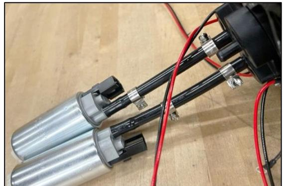
32. Using a 3/32" Allen wrench, resecure the brackets to the fuel hat, as shown.
