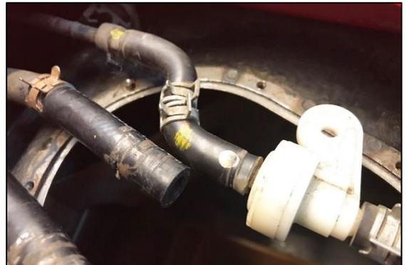
43. Rotate the rubber vent hose 180 degrees and secure with the spring clamps, as pictured.
