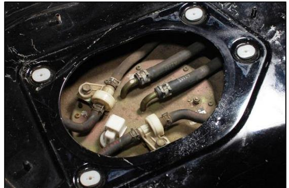
3. Before proceeding, it is recommended to clean the top of the fuel pump housing and the surrounding area. This will prevent loose dirt from falling into the gas tank.
