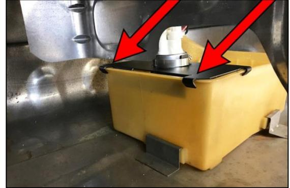
46. Next, gently squeeze the side walls of the OEM sub tank to allow the 2 baffle tabs to lock in place.
