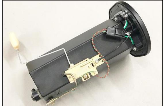
51. Move the FST assembly very close to the gas tank opening.
