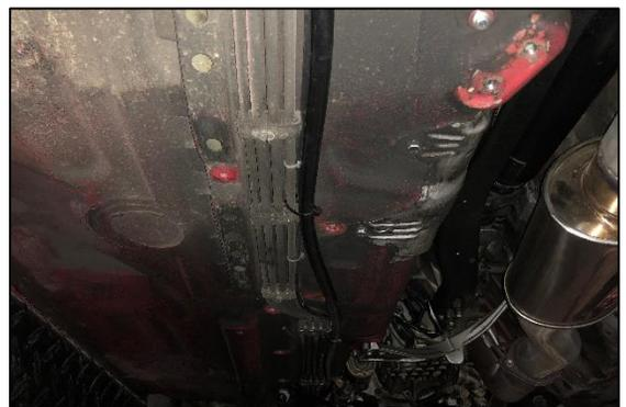
11. The feed line will route up into the engine bay where it will need to be connected to the fuel rail system of the engine. The exact details of this will depend on the engine and fuel delivery setup.
