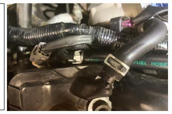
Install the provided plastic  ${\cal H}''$  to  ${\cal H}''$  90 degree elbow into the top portion of the 3-way junction. Point it directly upwards.
