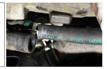
Route this 3/8" hose toward the top port of the rearmost catch can. Cut the 3/8" hose for best fitment. Ensure the hose is not kinked or pinched.
