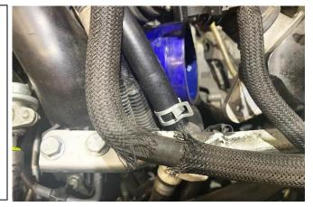
Run the  $\frac{1}{2}$ " hose towards the included TEE fitting and cut to length. Using oil lubrication install the hose to the TEE fitting, as shown. Hose clamps are NOT required for the TEE fitting barbs.
