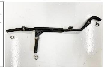
After unplugging the secondary injection connector, you will find the 3-way junction behind the intake manifold. This includes the crankcase vent which send vapors to the turbo inlet pipe as well as the PCV valve which routes vapors to the intake manifold. NOTE: The diagram shows how the PCV system works from the factory (not with the catch can installed).
