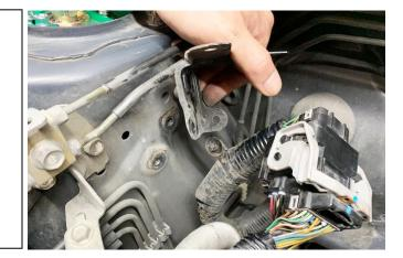
Unlatch the grey lock on the engine harness connector.
