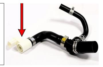
For aftermarket turbo inlets that do NOT support the OEM diagnostic connector, extra parts may need to be purchased. All that matters is that this port on the turbo inlet must be blocked off or plugged in some manner.
