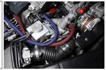
Cut a ½" section out of the hose shown. This cut should be made just behind the coolant tank. Next, install the provided TEE fitting in line with the branch of the TEE pointing toward the throttle body.
