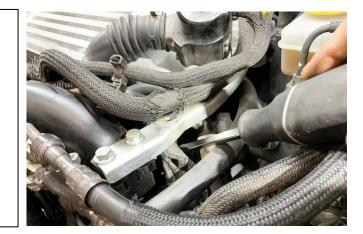
Move the intercooler back and forth to dislodge. Do not lose the turbo outlet gasket on the intercooler inlet. Carefully pull the intercooler upwards and remove from the vehicle.
