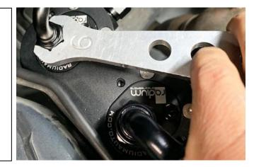
Attempt to slide the heat shield into position. Depending on the vehicle, there is a chance the power steering hose may be contacting the heat shield. If this is the case, the OEM bracket will need to be tweaked slightly for added clearance.
