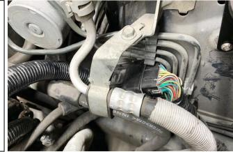
Using the two supplied M6x1mm socket head bolts and a 5mm Allen Wrench, secure the billet mount directly to the RH strut tower, as shown.
