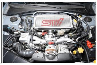
Find the large engine harness on the RH strut tower. The large connector will first need to be separated from the mounting bracket. Using a flat blade, simultaneously push the internal locking tab and pull apart to separate.
