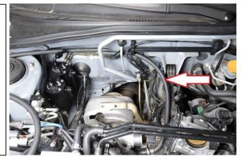
Using oil lubrication, install the 90 degree PushLok hose end into the 3/8" hose until all barbs are fully engaged. NOTE: clamps are not necessary for PushLok hose ends.
