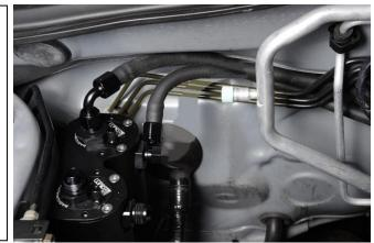
The 5/8'' barb found on the 3-way TEE (shown) will be converted to 1/2'' to be compatible with the 8AN hose end fittings. One short 1/2'' hose will be constructed.
