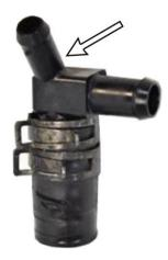
Reinstall the recirculation hose back onto the turbo air inlet pipe and route it as it was originally.
