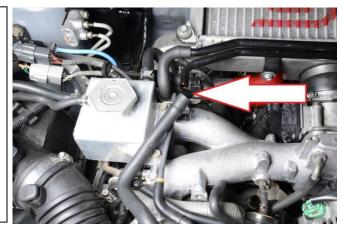
Connect one end of the provided ½" hose to the crossover tube. Next, route the hose over to the 90 degree hose end on the top port of the catch can. Cut the hose to length and install onto the hose end, as shown in blue. NOTE: Push Lok hose ends do NOT require hose clamps.
