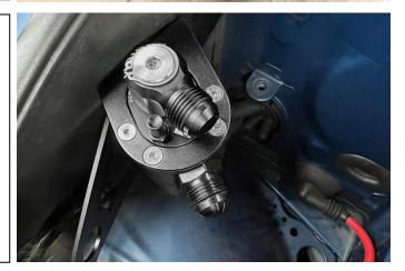
5. The factory crankcase vent tubing routes from the valve cover to the OEM AOS. The catch can hoses will be plumbed between these two connections.
