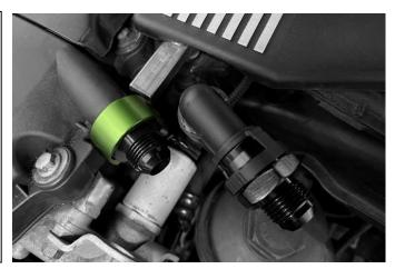
9. Next, the catch can hoses will need to be routed through the compartment wall into the engine bay.
