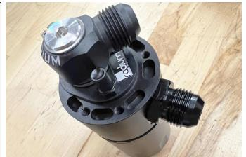
4. Confirm the catch can's bottom port is plugged or close the optional petcock valve, if applicable.
