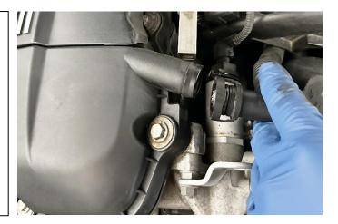
6. The next step will be rotating this connector around 180 degrees with respect to the tubing.
