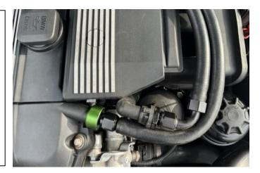
13. At the catch can, temporarily screw on each straight hose end.
