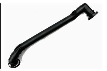
7. Carefully rotate the hose end fitting shown. This is the end of the tubing that connects to the valve cover. Oil lubrication can help.
