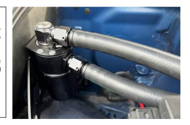
14. As shown, use the provided cable zip ties to secure the hoses together. Prior to closing the hood confirm there is adequate hood clearance.
