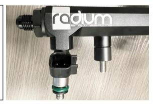
9. Place the fuel rail assembly onto the intake manifold. Push the injector lower O-rings into their respective injector seats.
