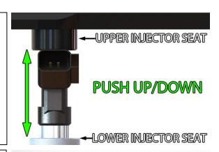
11. Orientate the fuel injectors such that the electrical connectors do not experience any interference with the surrounding area.
