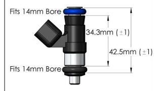
8. Lubricate the top and the lower fuel injector O-rings with engine oil.
