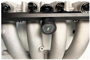
10. As a test, push the fuel injectors downward until they bottom out. Now inspect the injectors' upper O-rings and confirm they are still inserted into the fuel rail injector bores. Do not pressurize the fuel system until the proper height is achieved.
